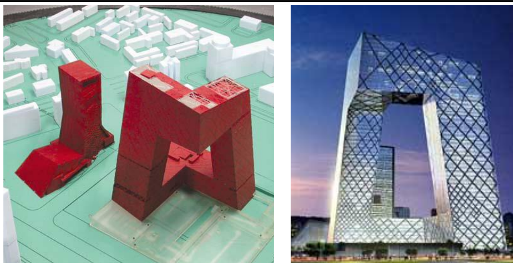
Figura 4-1: China Central Television Headquarters – Modelo em Túnel de Vento e fotografia (Xie & To, Design-Oriented Wind Engineering Studies New China Central Television Headquarters, 2008)
