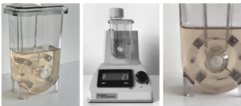
Figure 4.3. Vertical-wheel bioreactor PBS Mini 0.1L by PBS Biotech. Vertical-wheel bioreactors are designed for single use and ensure a consistent culture environment through gentle and efficient stirring. These bioreactors employ a large vertical wheel to achieve radial and axial mixing, while the U-shaped bottom prevents dead zones and limits cell settling. This design allows for lower agitation speeds, reducing shear stress on cells. Magnetic coupling between the impeller's magnets and the base unit drives the agitation, resulting in effective and gentle mixing.
