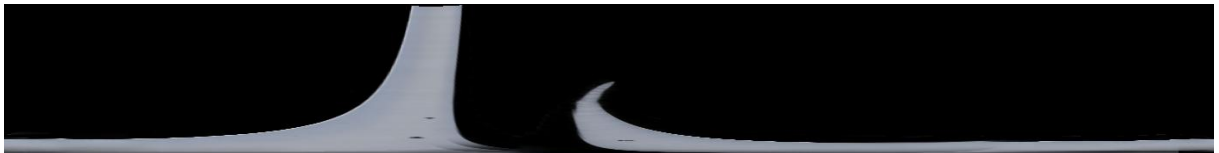
Figure 5.3: Autostitch software result having as input the entire dataset of the low-pressure side of the blade. The same input given to the tailored made solution.
