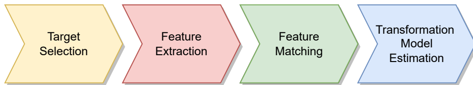
Figure 2.4: Flow diagram of a general image registration process, outlining the four steps: (1) Target Selection; (2) Feature Extraction; (3) Feature Matching; and (4) Transformation Model Estimation.
