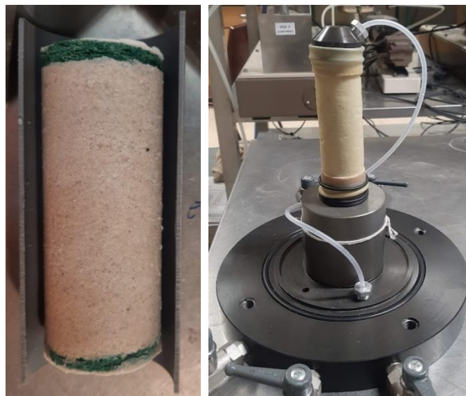
Figure 4.11 – Demoulded sample after biocementation treatment (left) and (right) sample on the triaxial equipment (right)
