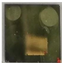
Figure 3.20 – Gold pad assay with a visible positive signal (the visible two white circles on top) and no spots indicating a negative signal (the absence of the two white circles on bottom).
