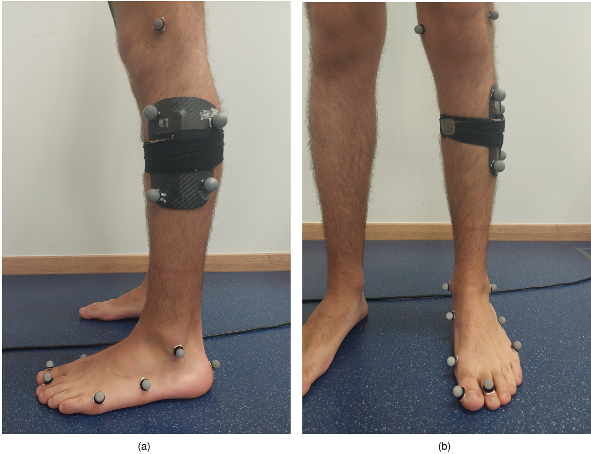
Figure 6.5: Positioning of reflective markers for the gait cycle trial: side view (a) and front view (b).
