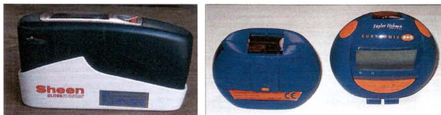
Fig 2 Photographs of the glossmeter (left) and the roughmeter (right)
