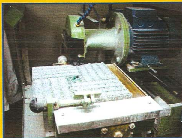
Fig.2 Detail of a grinding test. As it is possible to observe the surface of the stone is completely full of ground slots, for which the test is considered completed for this specimen
