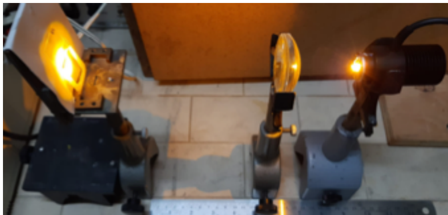
Figure 4.20 - Experimental setup used for irradiating samples with LED595nm. A lens was placed 3 cm from the source and a sample holder 12 cm from the lens.
