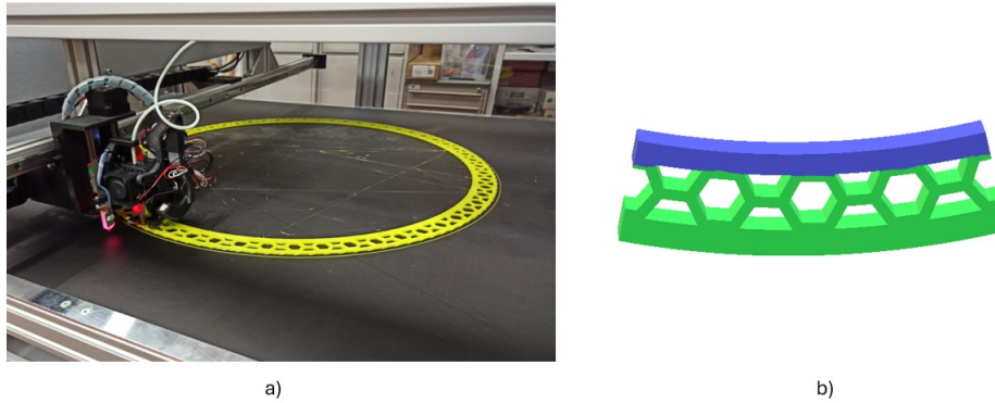
Figure 4.15: a) Single Piece (SM) tire being printed b) structure with TPU (green) and PLA (blue)
