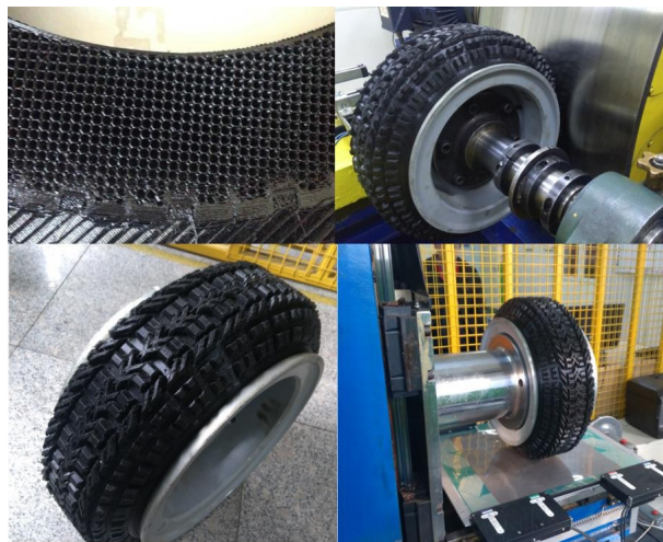
Figure 2.10: China's first 3D printed TPU tyre with FFF - 2017 [54]
