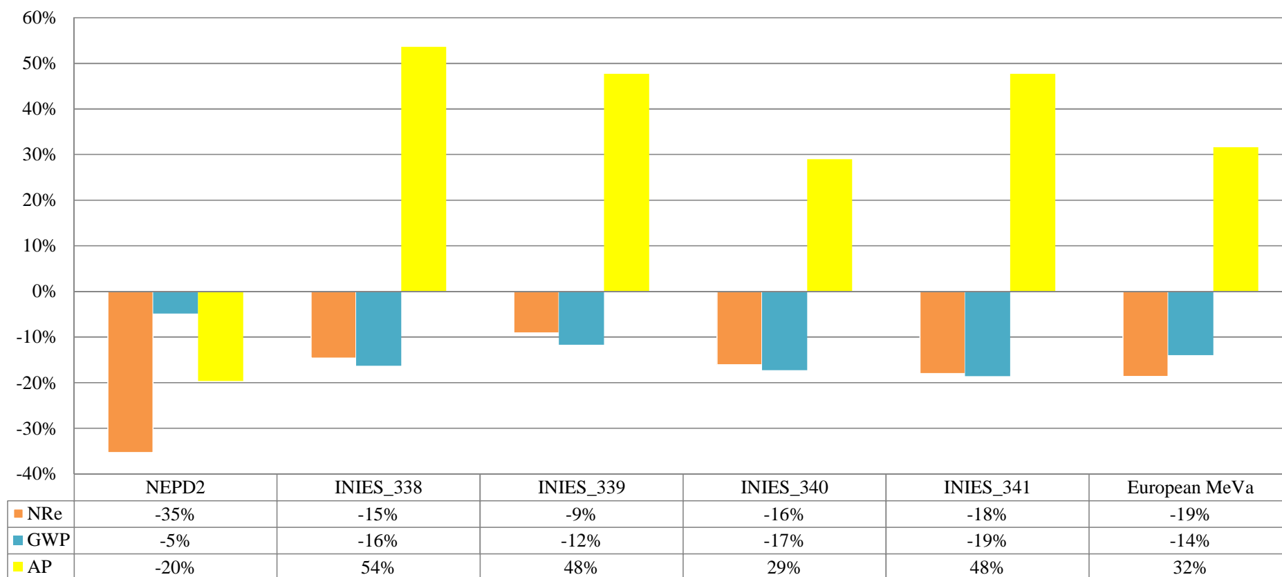
Figure 6.35 – Differences in PE-NRe (in orange), GWP (in blue), and AP (in yellow) in the production of one kilogram of gypsum plasterboard (A1-A3.3, including the packaging material) between national site specific data and individual EPD (Norwegian – NEPD, and French - INIES) and European MeVa
