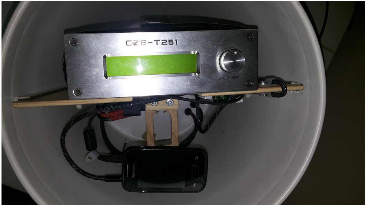
Figure 3.4: Image showing earliest RootIO transmission site devices (Android phone and Transmitter) housed in actual bucket
