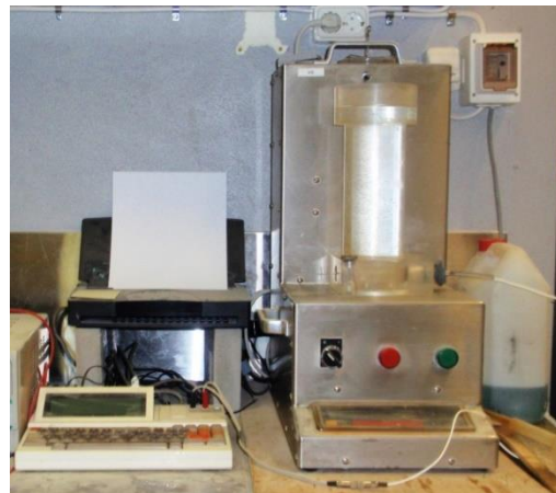
Figure 4.5 – AVA test set-up. Riser column with inverted pan on (on the right) and computer and printer that process the information (on the left).
