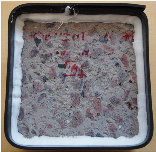
Figure E. 28 – Picture of specimen A, Mix 5 (50% GGBS, 6% Air, k=0.6 , carbonated), after 112 freeze/thaw cycles
