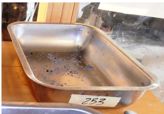
Figure 4.20 – Scaled-off material collected on a steel vessel.
