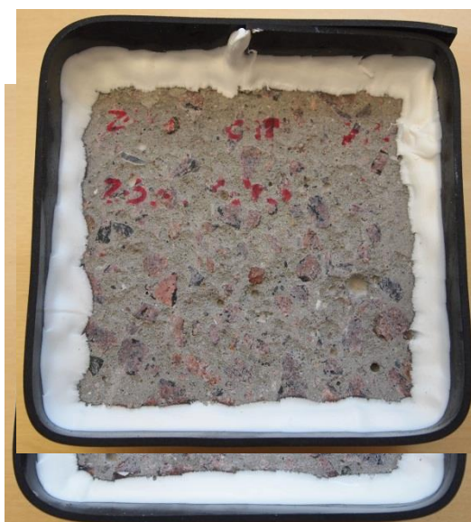
Figure E. 2 - Picture of specimen B, Mix 1 (0% GGBS, 4,5% Air) after 112 freeze/thaw cycles
