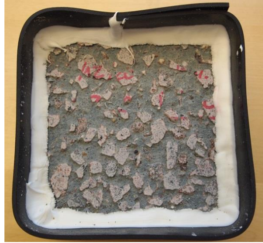
Figure E. 22 – Picture of specimen B, Mix 4(b) (100% GGBS, 4,5% Air, k=0.6 , cured at 55°C) after 112 freeze/thaw cycles
