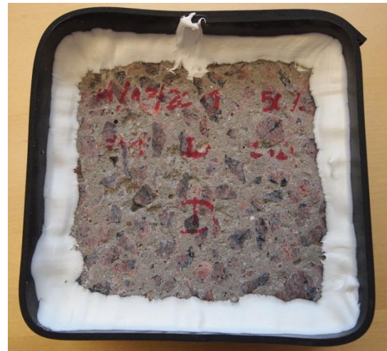
Figure E. 35 – Picture of specimen D, Mix 6(a) (50% GGBS, 4,5% Air, k=1 ), after 112 freeze/thaw cycles
