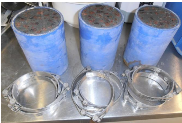
Figure 4.8 – Specimens for the Rapid Chloride Migration test fitted inside the rubber sleeve.
