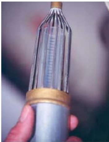
Figure 4.4 – Wire cage surrounding the syringe used to collect the sample for the AVA test [German Instruments (2009)].
