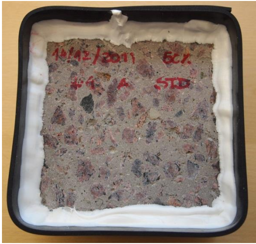
Figure E. 32 – Picture of specimen A, Mix 6(a) (50% GGBS, 4,5% Air, k=1 ), after 112 freeze/thaw cycles
