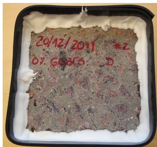
Figure E. 4 – Picture of specimen D, Mix 1 (0% GGBS, 4,5% Air) after 112 freeze/thaw cycles
