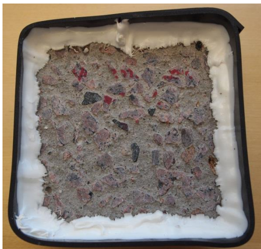
Figure E. 17 – Picture of specimen A, Mix 4(a) (100% GGBS, 4,5% Air, k=0.6 ) after 112 freeze/thaw cycles
