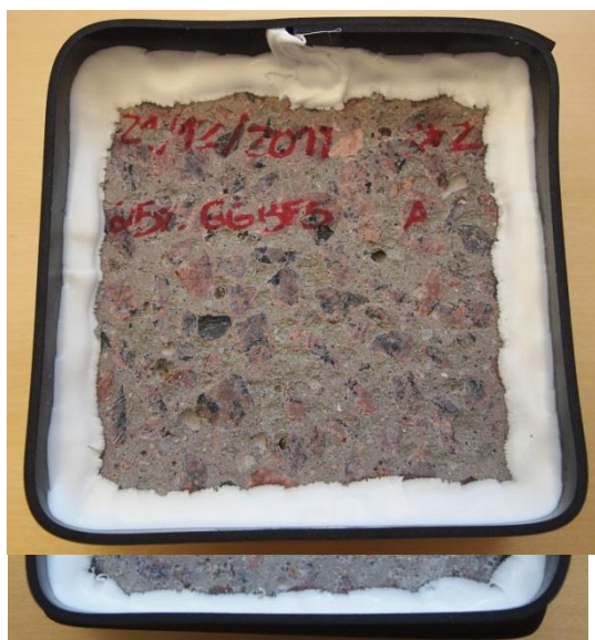
Figure E. 1 – Picture of specimen A, Mix 1 (0% GGBS, 4,5% Air) after 112 freeze/thaw cycles
