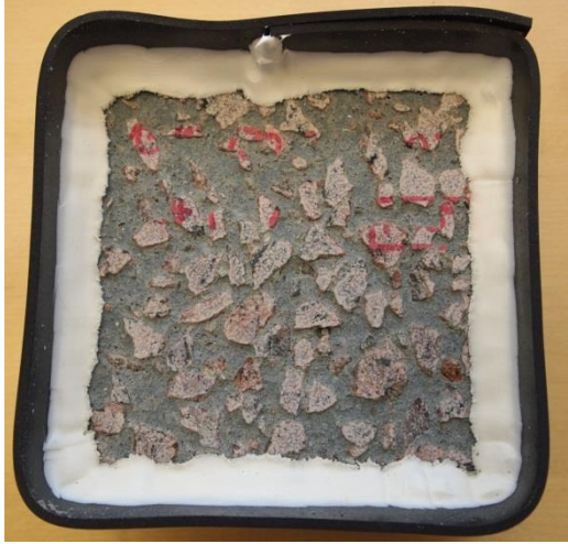
Figure E. 21 – Picture of specimen A, Mix 4(b) (100% GGBS, 4,5% Air, k=0.6 , cured at 55°C) after 112 freeze/thaw cycles
