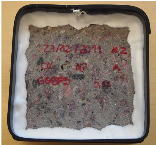
Figure E. 39 – Picture of specimen A, Mix 7 (0% GGBS, 4,5% Air, no superplasticizer) after 112 freeze/thaw cycles
