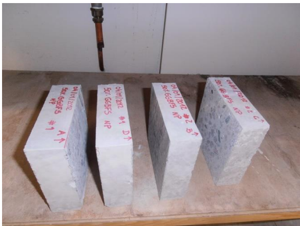
Figure 4.15 – Slab specimens pre-conditioned in the climate chamber.
