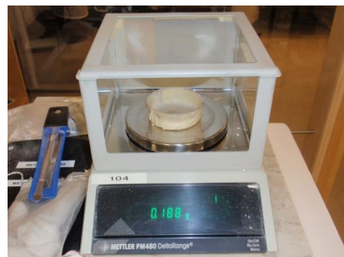
Figure 4.21 – Determination of the mass of scaled material.
