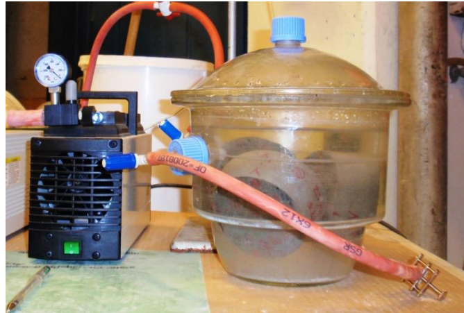
Figure 4.7 – Vacuum container holding the test specimens covered in the \text{Ca(OH)}_2 solution, after being disconnected from the vacuum pump.
