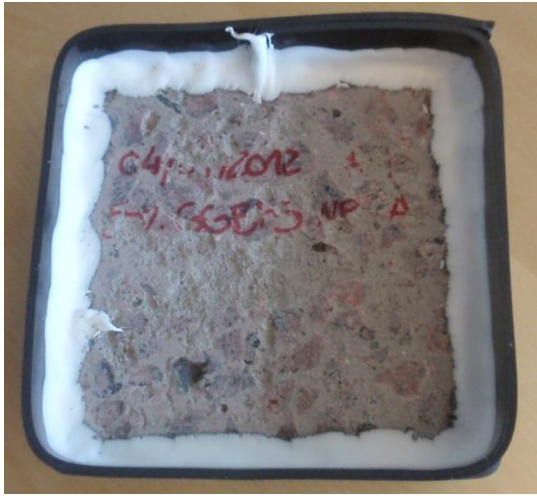
Figure E. 43 – Picture of specimen A, Mix 8 (50% GGBS, 4,5% Air, k=0.6 , no superplasticizer) after 112 freeze/thaw cycles
