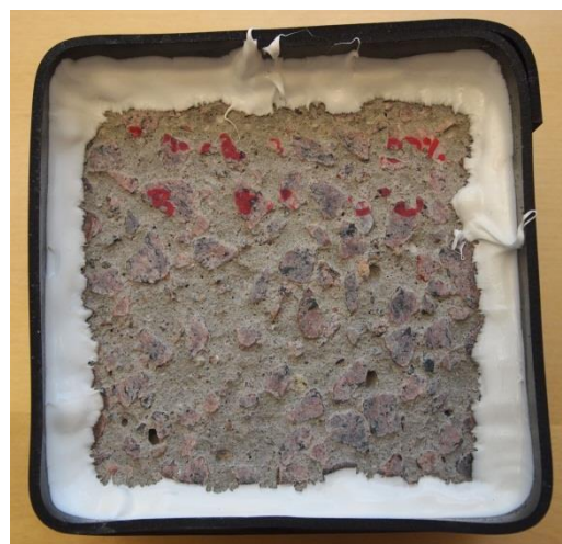
Figure E. 18 – Picture of specimen B, Mix 4(a) (100% GGBS, 4,5% Air, k=0.6 ) after 112 freeze/thaw cycles
