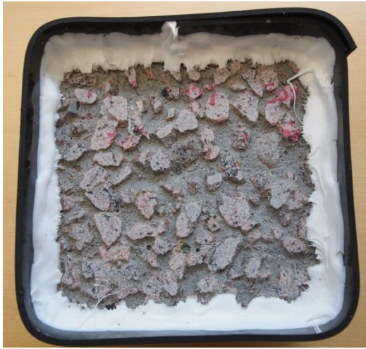
Figure E. 36 – Picture of specimen A, Mix 6(b) (50% GGBS, 4,5% Air, k=1 , cured at 55°C), after 112 freeze/thaw cycles
