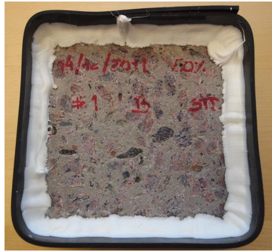
Figure E. 33 – Picture of specimen B, Mix 6(a) (50% GGBS, 4,5% Air, k=1 ), after 112 freeze/thaw cycles
