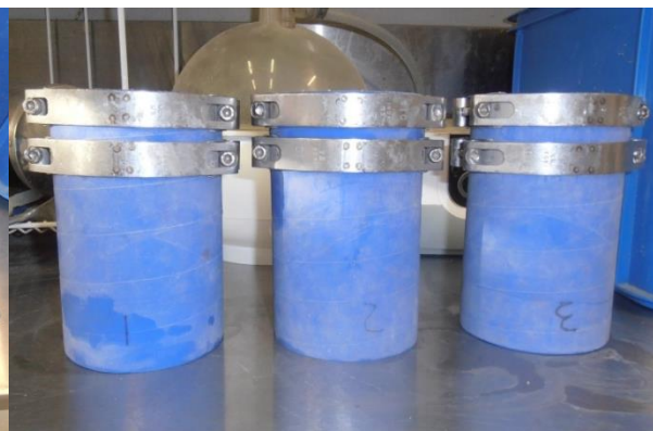
Figure 4.9 – Specimens for the Rapid Chloride Migration test secured with clamps to prevent leakage.
