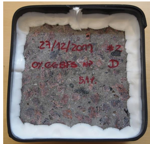
Figure E. 42– Picture of specimen D, Mix 7 (0% GGBS, 4,5% Air, no superplasticizer) after 112 freeze/thaw cycles
