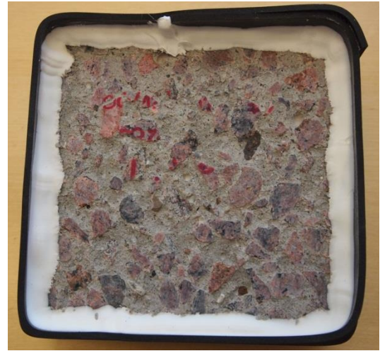
Figure E. 14 – Picture of specimen B, Mix 3 (50% GGBS, 4,5% Air, k=0.6 , carbonated) after 112 freeze/thaw cycles
