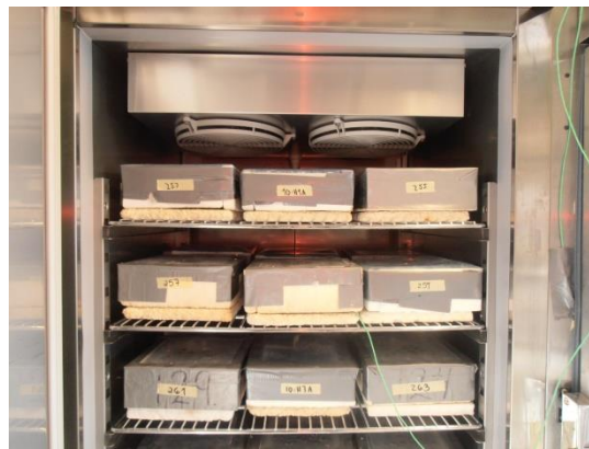
Figure 4.18 - Salt-frost scaling test specimens placed in the freezer.
