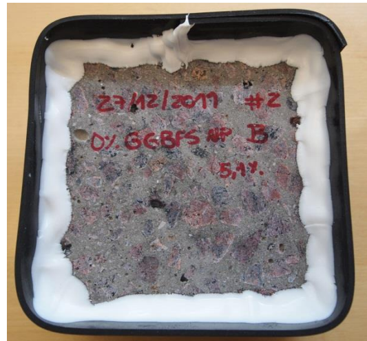
Figure E. 40 – Picture of specimen B, Mix 7 (0% GGBS, 4,5% Air, no superplasticizer) after 112 freeze/thaw cycles
