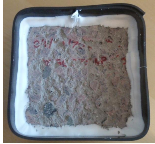
Figure E. 44 – Picture of specimen B, Mix 8 (50% GGBS, 4,5% Air, k=0.6 , no superplasticizer) after 112 freeze/thaw cycles
