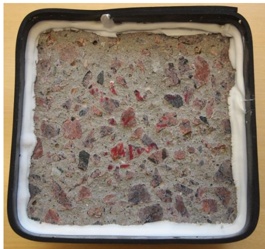
Figure E. 15 – Picture of specimen C, Mix 3 (50% GGBS, 4,5% Air, k=0.6 , carbonated) after 112 freeze/thaw cycles
