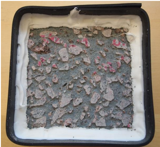
Figure E. 21 – Picture of specimen A, Mix 4(b) (100% GGBS, 4,5% Air, k=0.6 , cured at 55°C) after 112 freeze/thaw cycles
