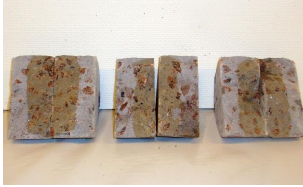
Figure 4.12 – Test specimens for the Rapid Chloride Migration test after being sprayed with silver nitrate solution.
