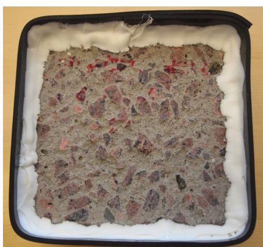
Figure E. 27 – Picture of specimen D, Mix 5 (50% GGBS, 6% Air, k=0.6 ), after 112 freeze/thaw cycles
