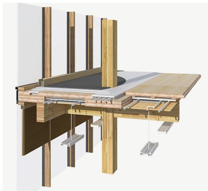
Figure 52. Wood structure and building enclosure elements of Wood Innovation and Design Centre (Wood Innovation and Design Centre, n.d.)
