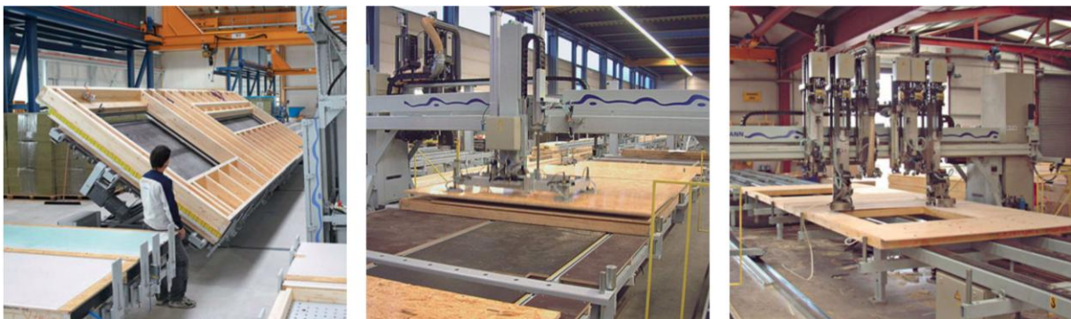
Figure 40. Prefabrication of an engineered timber panel (Kaufmann et al., 2018)
