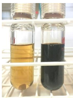
Figure 3 - Time zero of a reaction (MCR02), where reagent A gives the yellow color (left) and time seventeen of the same reaction (right)
