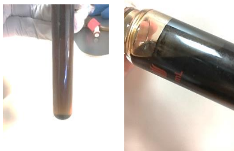
Figure 4 - Observation of by-products formation. On the left it is observed sedimented solids in the bottom of the tube. On the right it is observed precipitated at the walls of the high pressure vessel
