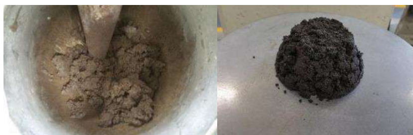
Figure 2 - Mortar using a polycarboxylate-based WRA
