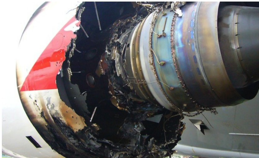
Figure 1.2: Rolls-Royce Trent 900 engine failure, Singapore, Changi Airport in 2010 [2].
