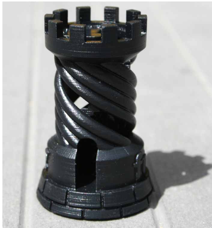
Figure 4.15: Soft surface in 25 \mu m resolution with SL technology.
