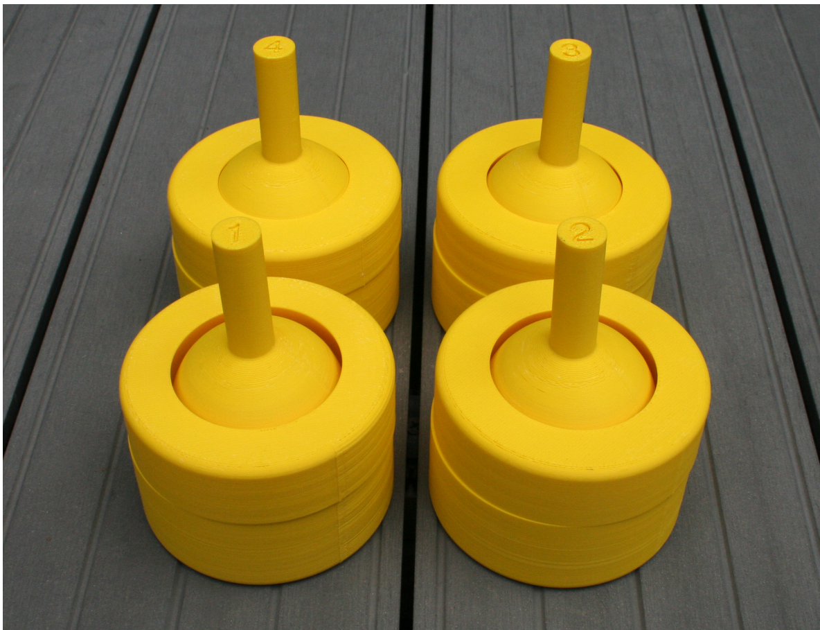
Figure 5.8: Parts already manufactured in ABS with the SST-768 in a 254 \mu\text{m} resolution.
