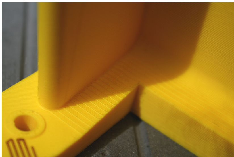
Figure 4.13: Visible rungs on a real FDM part with 254\mu\text{m} layer thickness
