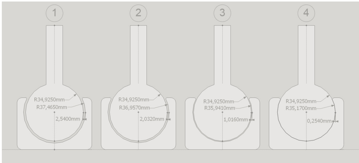
Figure 5.6: Ball and socket gap.
