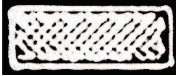
Figure 4.8: Non-filled area in a FDM cross-section.[34]
